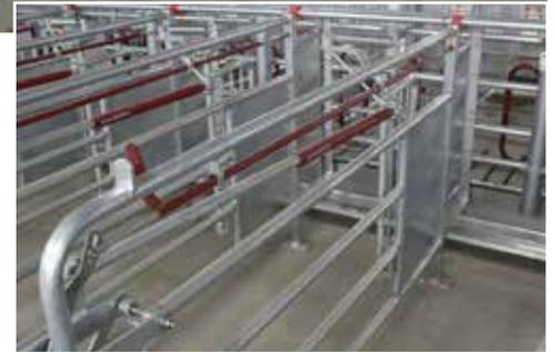
The connection rod between the front and rear gate on the Classic Free-Access Gestration Stall has an integrated spring helping to prevent injuries to sows and damage to gates.
