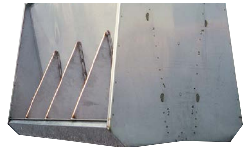
V-shaped bottom directs feed-clogging moisture away from the feed dispensing area.
